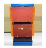
THE THICKNESS MEASURE OF THE FILM IS DONE BY COMPARING THE ABSORBANCE OF THE IR RADIATION AT DIFFERENT WAVELENGTHS (UP TO 11 — NEW )
