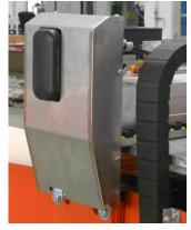
THE CAPACITIVE SENSOR IS A REFLECTION GAUGE ENGINEERED FOR THICKNESS MEASUREMENT. THE GAUGE BASES ITS FUNCTIONING ON CAPACITIVE TECHNOLOGY, IT FOUND ITS MAJOR APPLICATION IN BLOWN FILM OR DOUBLE BUBBLE PLANTS, INSTALLED IN A WAY TO MEASURE DIRECTLY ON THE BUBBLE, BEFORE THE COLLAPSING FRAMES.
