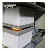
Sensor working similarly to **DIGILAYER** but with max 6 different wavelengts taken simultaneously and in same spot, that is a relevant feature in case of very not homogeneous film.
