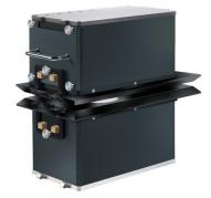
THIS SENSOR MEASURES THE SURFACE WEIGHT OR THICKNESS OF FLAT SHEET MATERIALS, USING NON-IONISING, ELECTROMAGNETIC WAVES FOR THE CONTACT-FREE MEASURING PROCESS. IT IS SUITABLE FOR ACCURATE AND RAPID MEASUREMENT OF POLYMER-BASED MONO AND MULTILAYER FILMS.
