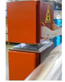
In case the film is very thick and rigid and cannot wrap around a roll, it can be used a double ESSAIR sensor. Each sensor measure its distance P1 and P2 from the top and bottom surface of the film, the distance M1 between the two ESSAIRs is measured by one of the inductive sensors. The thickness is calculated from these values.
